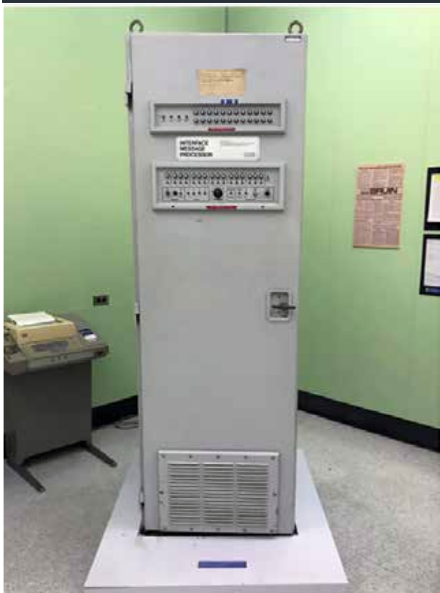
The Interface Message Processor (IMP) functioned as the internet's first router
